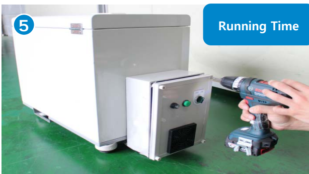
Running time is 5 mins. If you want to change, loosen 4 volts.
