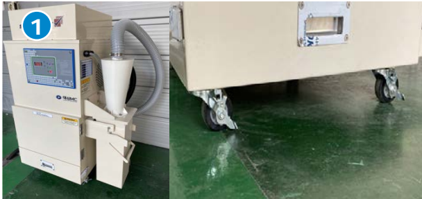
Fix the wheels to place the dust collection box.
