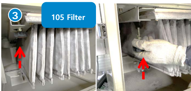
Loosen the four edge fixing screws.
