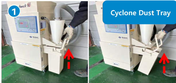
After turning off the power, lift the handle and discard the cyclone dust bin.
