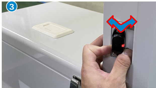
Set the sensor angle by turning left and right according to the site.
