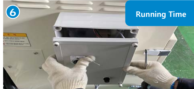
If you want to change the suction time, turn off the power and open the control box.
