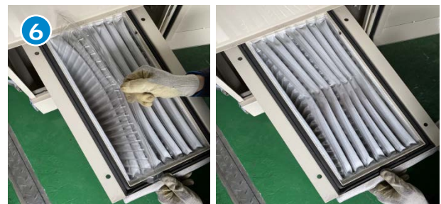
Put the air cap between the new filters. Assemble in reverse order.
