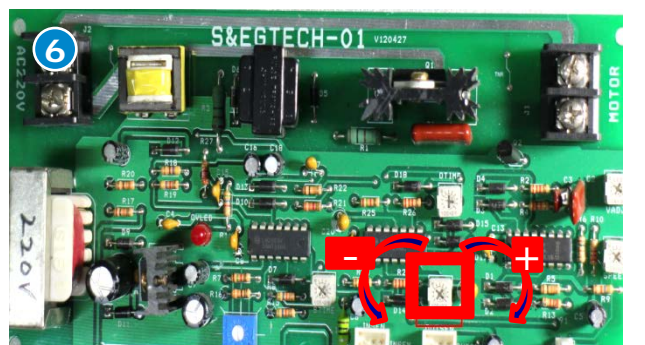
Set the Running Time. (Normally 5 sec.) (min.1 ~ max. 23 sec.)
