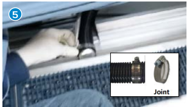
Tighten the hose with joint.
