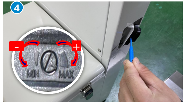
Set the sensor range according to the site. (Range : 0m-2m)
