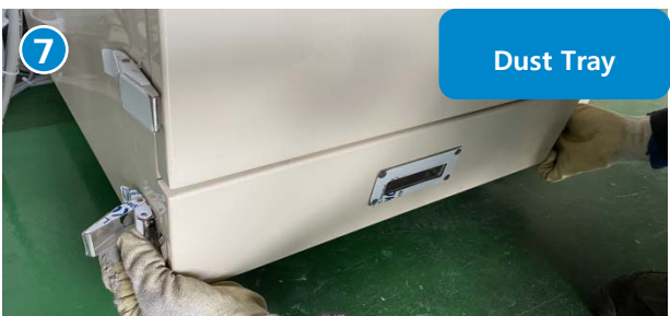
Open the hooks on both sides of the dust tray below.
